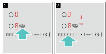
The function has now been activated. The **1** temperature symbol will remain lit until the frying temperature has been reached. An audible signal sounds and the temperature symbol goes out.
